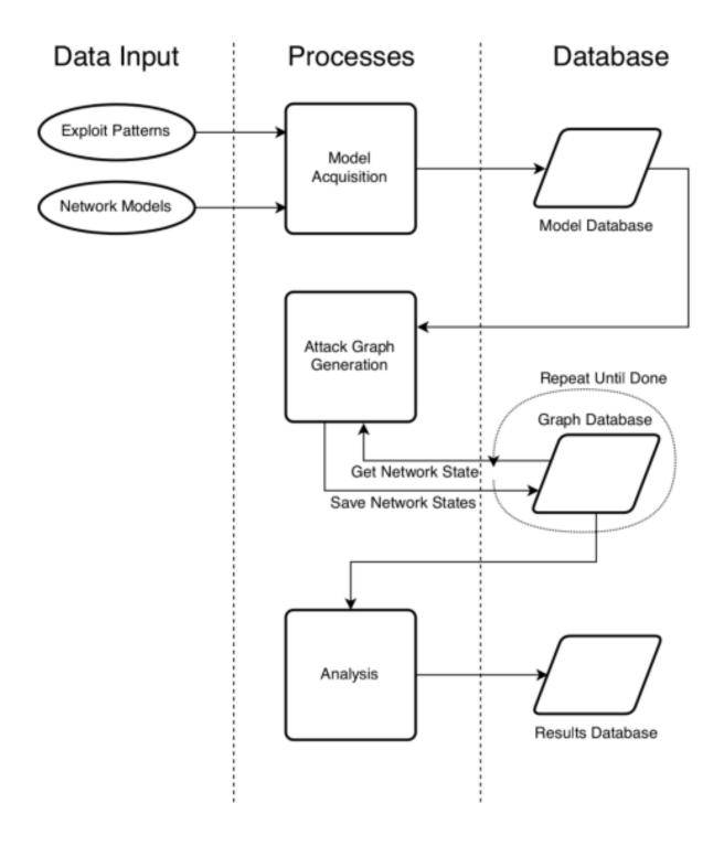
Figure 5.1: Generation Flowchart of RAGE
